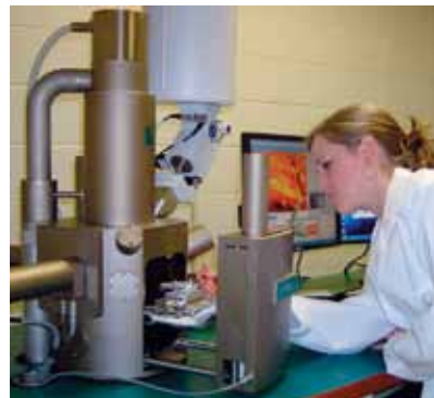
High-resolution scanning electron microscopes (above) and other devices are used to evaluate metal structures—often to determine the cause and prevention of product failure.
